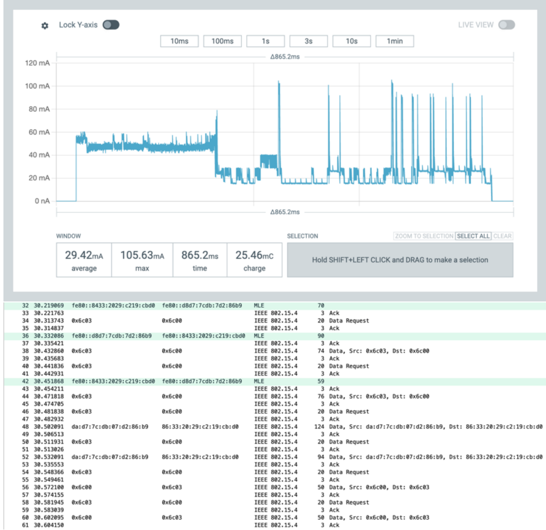
Figure C.3: The energy consumption of a SED for a single wakeup when packets are secured under ASCON-128a, and when operating with the TX power of 20 dBm.
