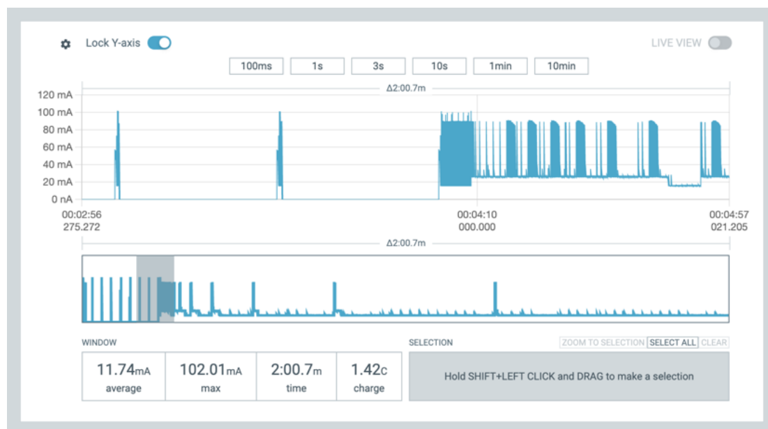
Figure A.21: SED (3) did not go to deep sleep when it had network connection issues in the initial run of the ASCON-128 20 dBm experiment. The minimap is shown to highlight that SED (3) never went into deep sleep. Furthermore, timestamps are shown to note that SED (3) had a network connection issue 4 minutes into the experiment.
