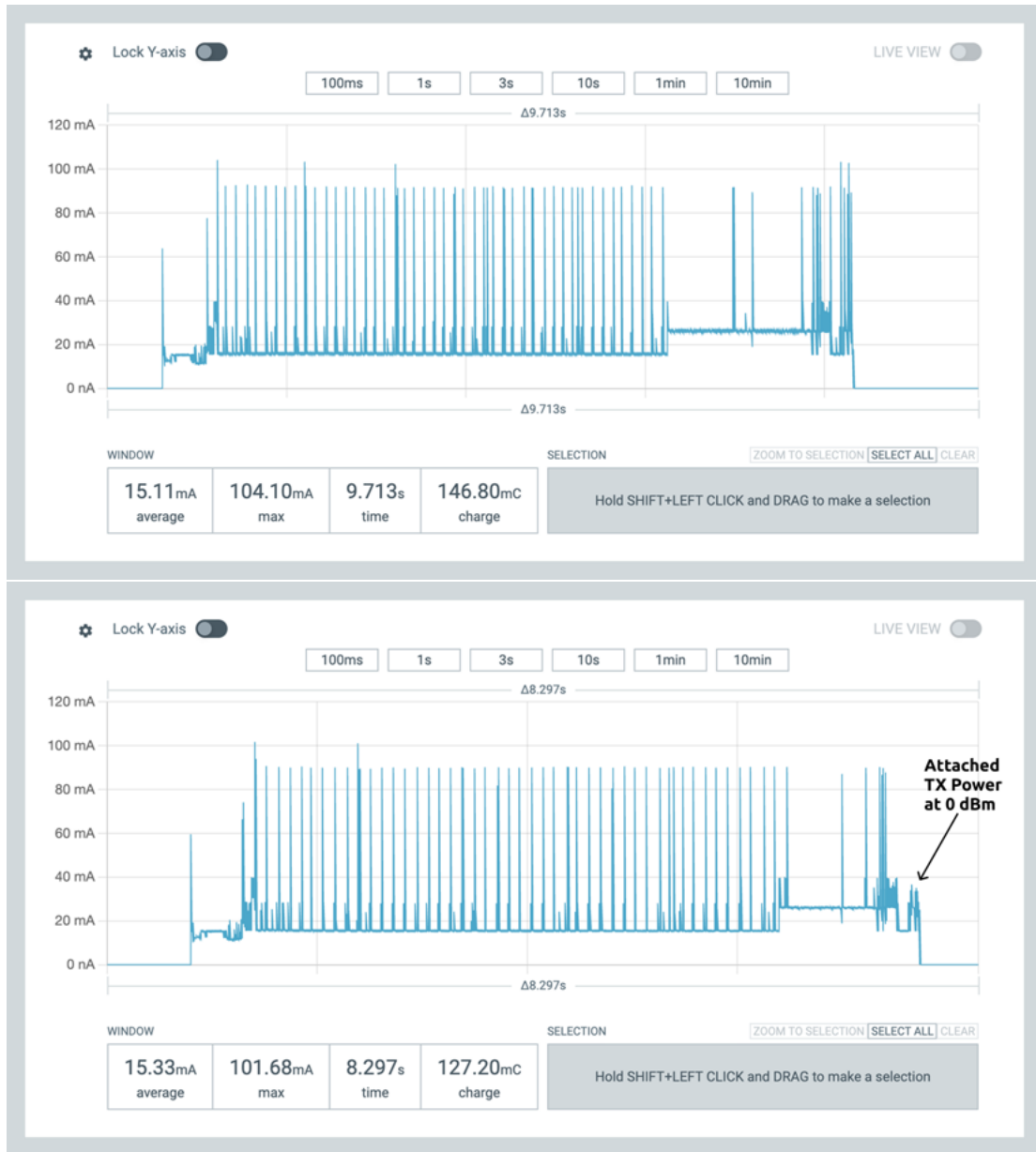
Figure A.20: The waveforms of SED (3) when first powering on, during the AES-CCM 20 dBm and 0 dBm experiments are shown at the top and bottom, respectively.
