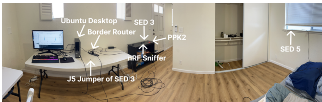
Figure 4.9: The experimental setup for the Energy Consumption experiments. SED (4) is not show in this picture, as it is hidden behind the wall past the door.
