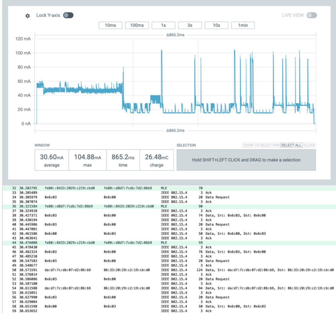
Figure C.4: The energy consumption of a SED for a single wakeup when packets are secured under ASCON-128, and when operating with the TX power of 20 dBm.
