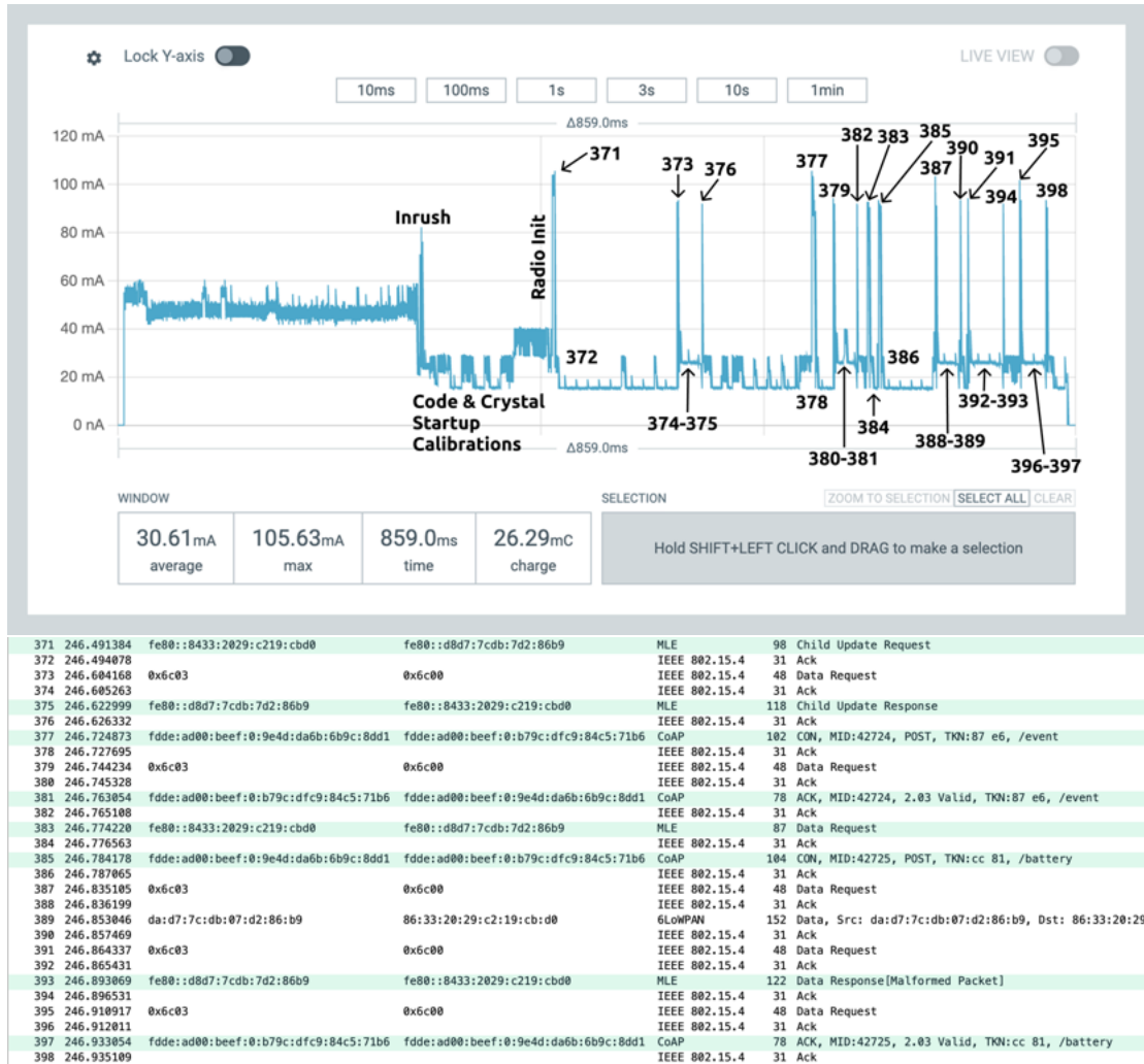
Figure 5.4: The energy consumption waveform 2 for a SED during a single wakeup, along with the corresponding Wireshark packet capture.
