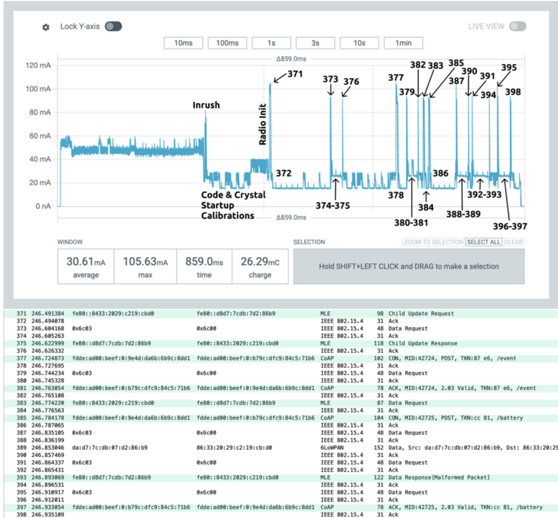
Figure C.1: The energy consumption of a SED for a single wakeup when secured under AES-CCM, and operating with the TX power set to 20 dBm.
